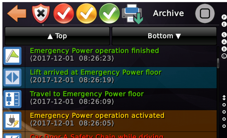
Figure 151: Logbook items for Emergency Power Operation
