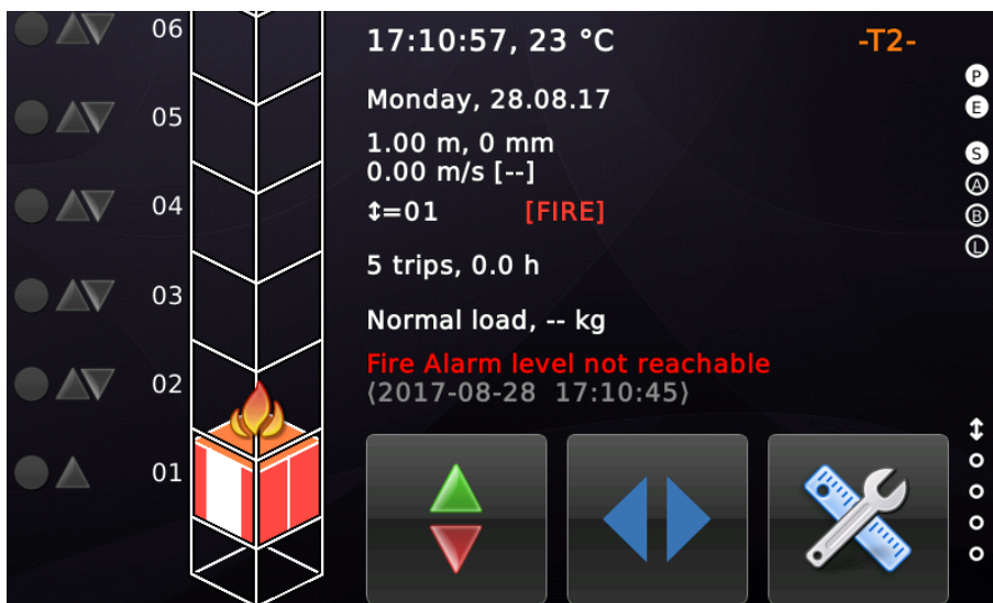
Figure 142: Fire Alarm level not reachable
