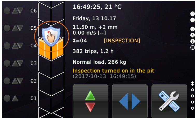
Figure 8: Lift waiting for inspection pit reset
