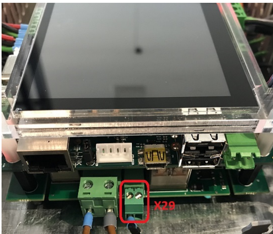
Figure 212: I/O SZ-Board – Terminal X29.
