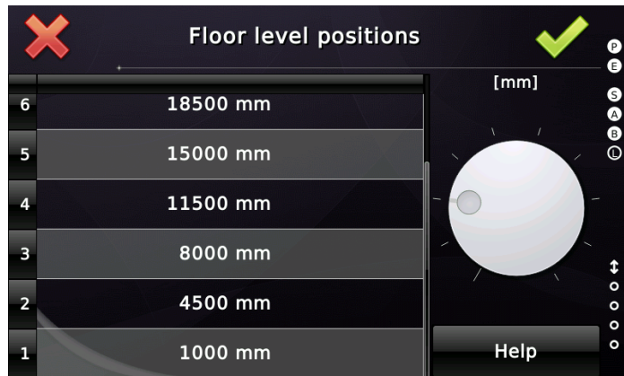
Figure 65: Floor Level Table
