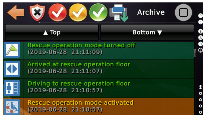
Figure 148: Rescue/Salvage operation mode recorded by the logbook
