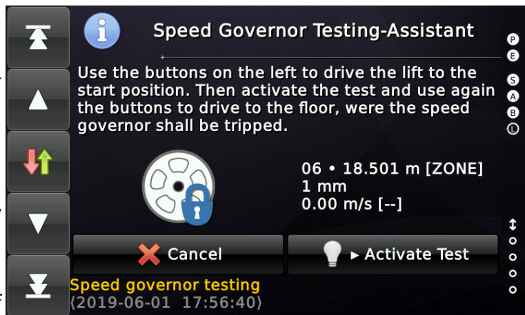
Figure 110: Speed Governor (SG) Test-Assistant
