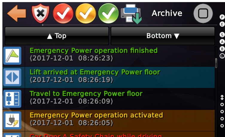
Figure 152: Logbook items for Emergency Power Operation
