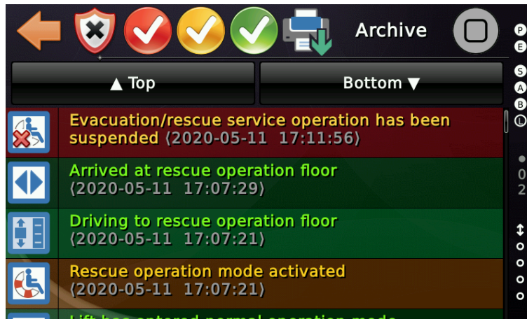
Figure 149: Evacuation operation suspended via an input signal
