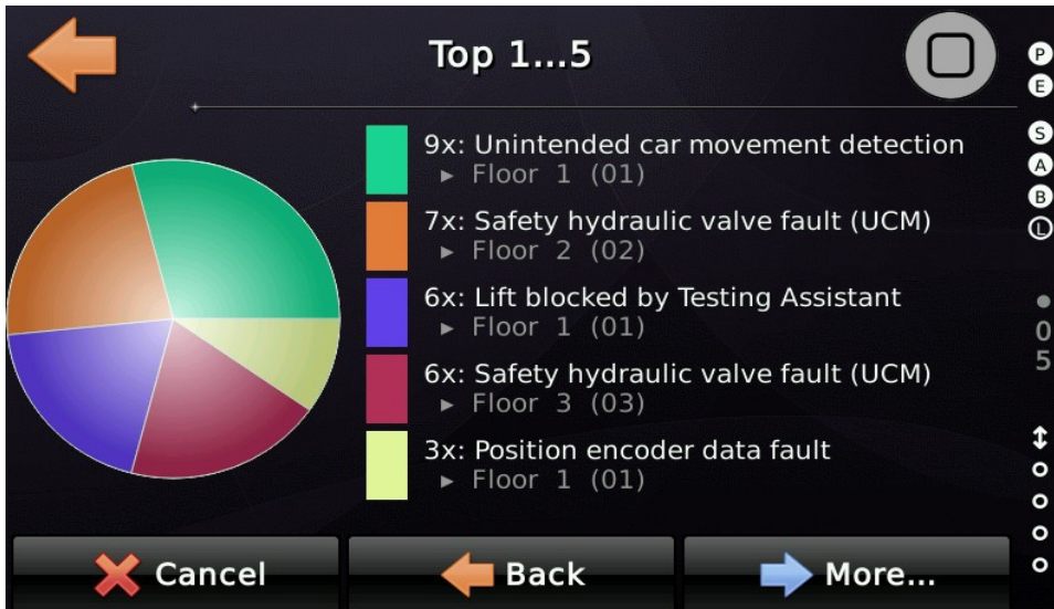
Figure 22: Pie chart showing the top 5 faults
