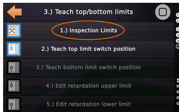
Figure 43: Teaching the inspection limits
