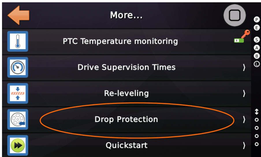
Figure 128: Menu path to the Drop Protection options
