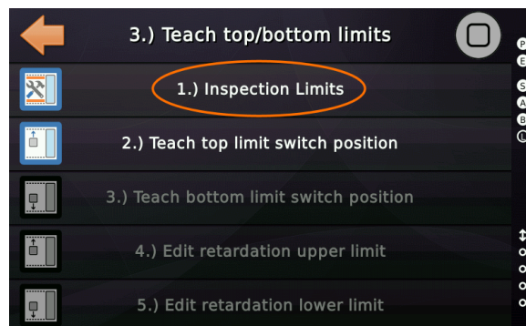
Figure 36: Teaching the inspection limits
